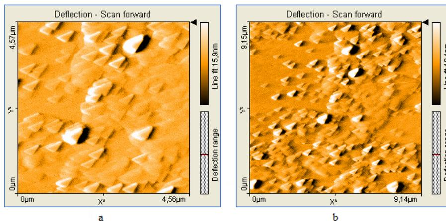
The 3D AFM image presented in Figure 7 outlines the formation of superposed triangular structures, corresponding to sandwich H-type aggregates, with dimensions ranging in the 370-480 nm domain.
