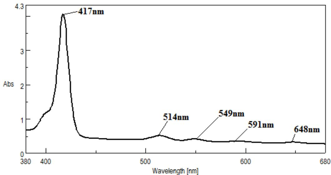
**Figure 3:** The superposed UV-vis spectra of the THF-water solution of the hybrid material at increasing CO<sub>2</sub> concentration
