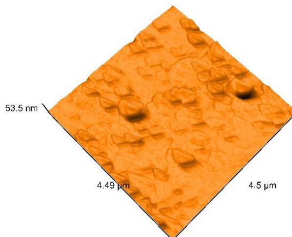
Particle analysis offer information about the mean surface of islands, that is  $0.0206 \mu\text{m}^2$ . The particles have a mean height of 0.8 nm, but the highest peak is around 40 nm. The mean rugosity is of 3.9 nm.
